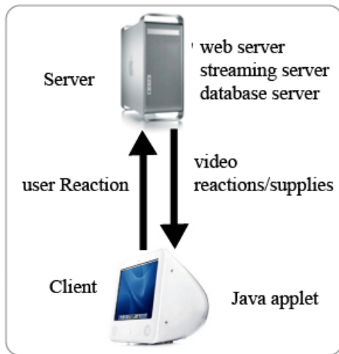
Figure2: System Diagram of the iPlayer
